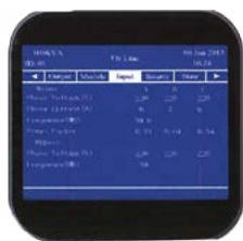
UPS Cabinet Control Panel
