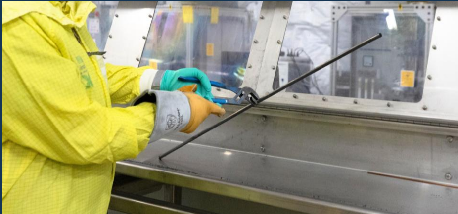
Uranium-Zirconium Rod Post-Extrusion
