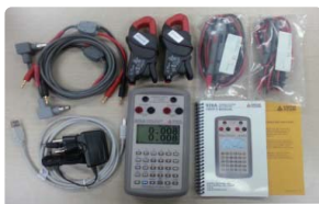
Power System Multi meter/ Angle Meter ARBITER [928A]
