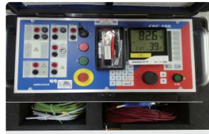
CT & PT Test Equipment (CPC-100)
