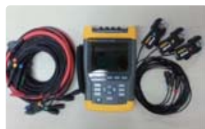
Power Quality Analyzer FLUKE [435]
