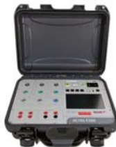
Circuit Breaker Test & Analyzing
