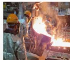
Workers are pouring molten metal in our factory to make casting material.
