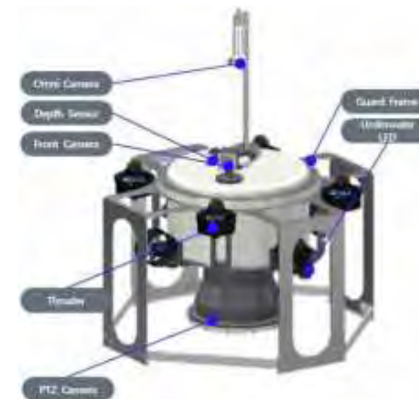
Intake Sediment Measurement Underwater Drone (ISMUD)
