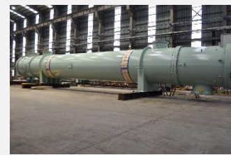
CCW Heat Exchanger for Akkuyu NPP
