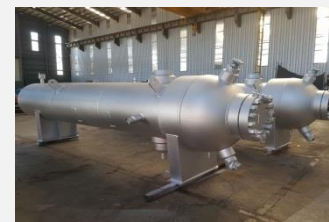
Fuel Gas Heater
