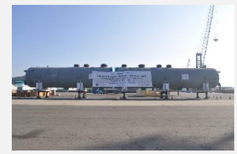
Deaerator & FWST for Akkuyu NPP
