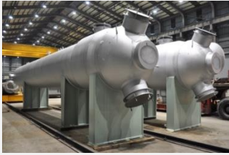
H.P. Feed Water Heater
