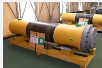
Lube Oil Cooler
