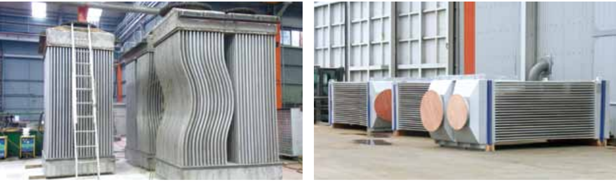
A. Use : 250 tons / hr Reheating Furnace B. Material : SICROMAL 12, SICROMAL 10, DIN 1.4720 C. Design temp. : 900°C D. Size(W x L x H) : 1,625mm x 2,650mm x 4,390mm E. Weight : 8,812 tons
