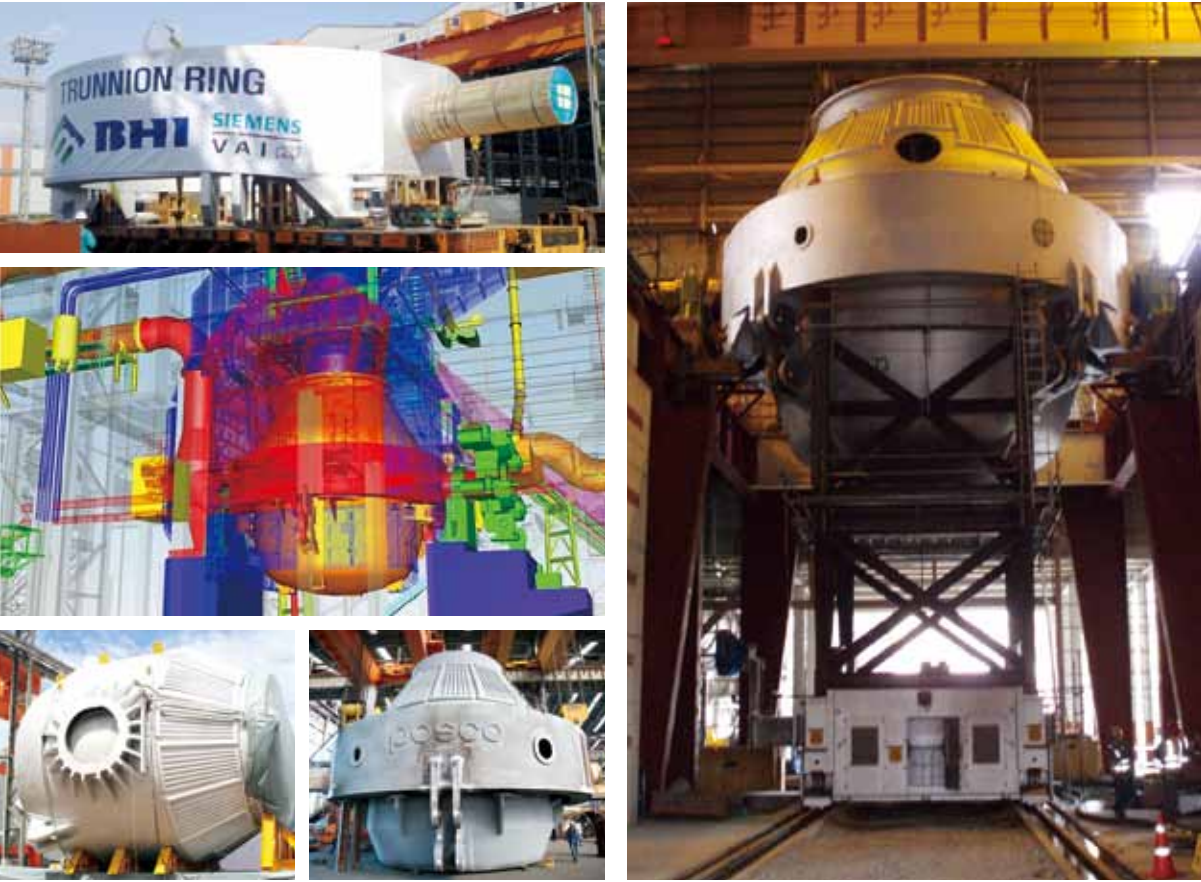
A. Material : STB340H B. Size(L x W x H) : 12,200mm x 5,200mm x 5,500mm C. Temp. : 235.5°C D. Weight : 580 tons E. Thickness : 180mm
