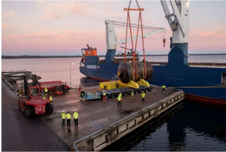
FIG. III–7. Shipping of EDF Fessenheim PWR NPP Steam generators from France to EDF-Cyclife Facility in Sweden (Courtesy of Cyclife-EDF, France).
