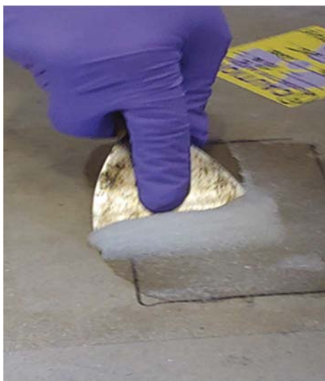
FIG. 17. SuperGel application to a contaminated surface (reproduced from Ref [55] with permission courtesy of CEA, France).
