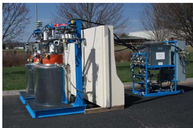
FIG. 11. Drum Dryer for Mop Water to Prevent Fouling Floor Drains. (Courtesy of Pacific Gas & Electric Company, USA).
