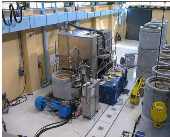
FIG. 23. Volume reduction of spent ion exchange resins before processing - Mercure process (Courtesy of EDF, France).
