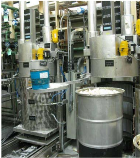
FIG. III–9. In-drum Drying System to reduce resin volumes before processing at Krško NPP. (Courtesy of Nuclear Safety Administration, Slovenia).
