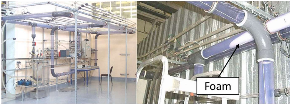
FIG. 20. Using foam technology for pipes decontamination (reproduced from Ref [56] with permission courtesy of CEA, France).
