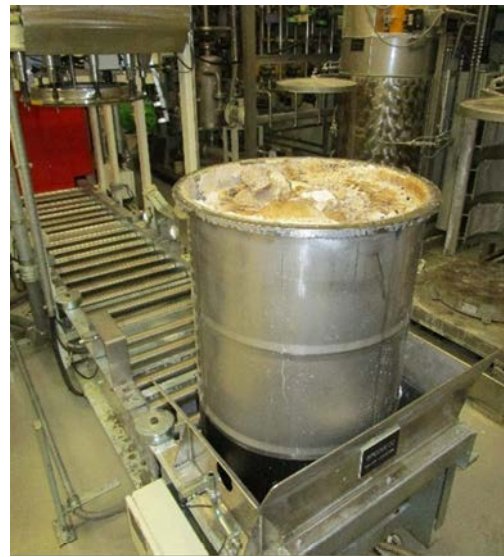
FIG. III–9. In-drum Drying System to reduce resin volumes before processing at Krško NPP. (Courtesy of Nuclear Safety Administration, Slovenia).
