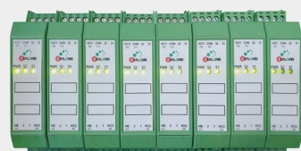
OPTO-COUPLER MODULE for ESFAS (Engineering Safety Features Actuation Signal)
